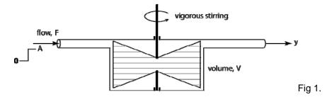
A simple model of concentration changes within a fluid pool is shown in Fig 1. A step change in concentration from zero to A has occurred at the input at t = 0.
